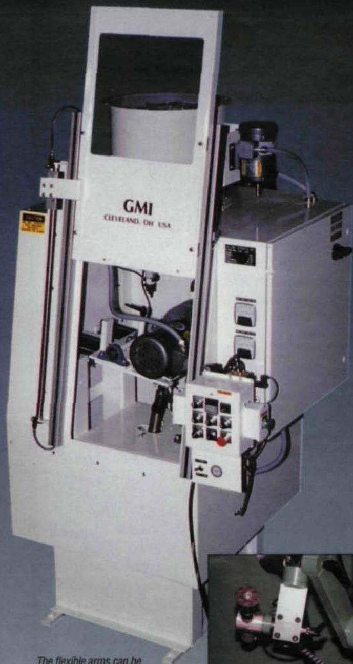
*The flexible arms can be fitted with conventional grinding wheels, CBN, pencil grinders, or milling attachments, for maximum versatility. Machines can also be furnished with electric motors (shown above) for brushing operations.*
