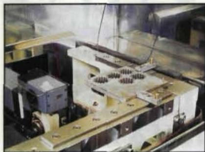
Fig. 3 — Stacked spur gears in an EDM.
