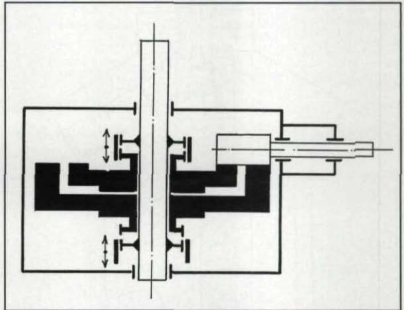
Fig. 10 — Ninety degrees ( $90^\circ$ ) dual-speed gearbox.
