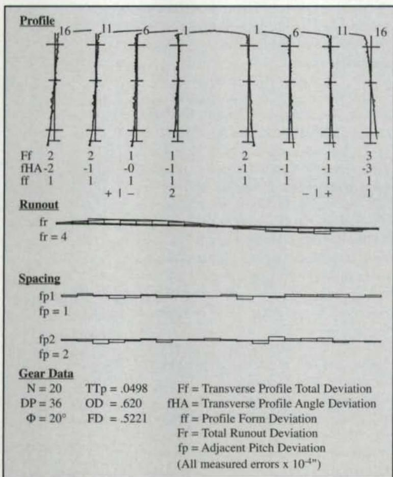
Fig. 7 — 36 DP wire EDM gear data.
