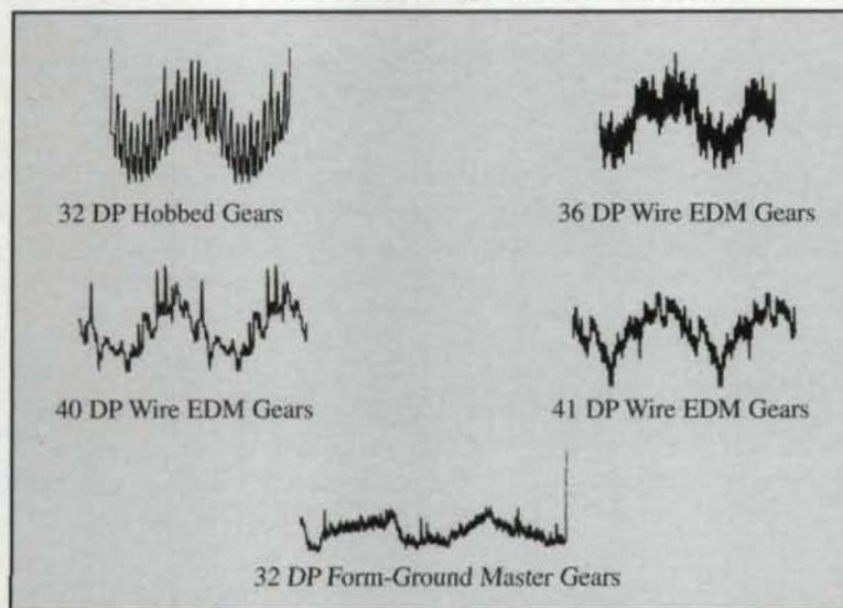
Fig. 10 — Roll tests.
