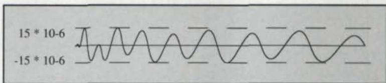
Fig. 5 — Deviation between splined arcs and involute.
