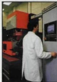
*Precision machines, both on and off the track, contribute to Formula One success. Above, the Marlboro-McLaren car with drivers. Below, the Charmilles wire EDM machine used to make transmission gears.*
