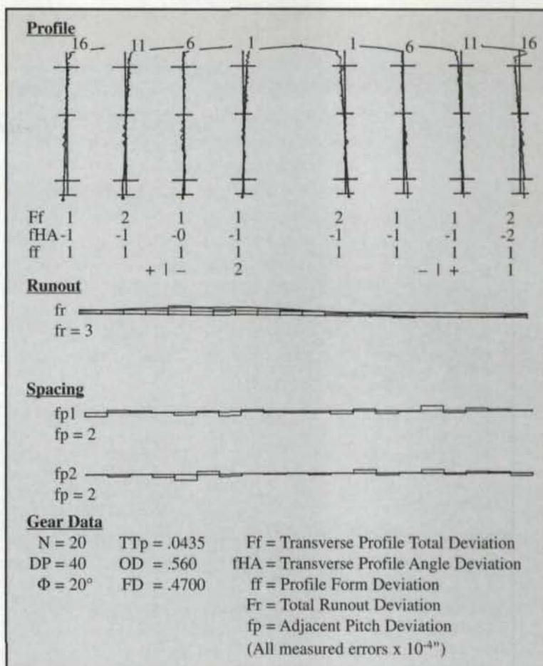
Fig. 8 — 40 DP wire EDM gear data.
