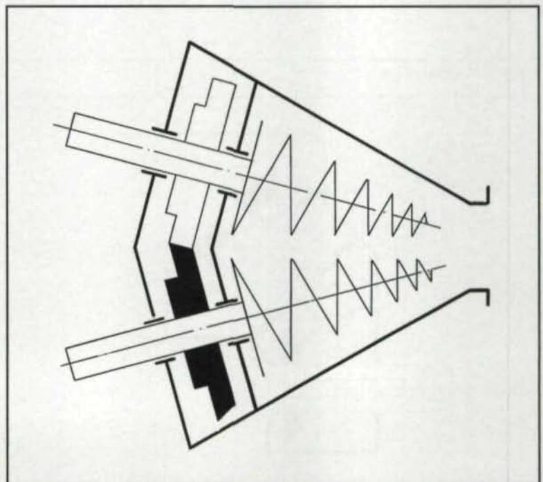
Fig. 11 — Dual-feed screw for an injection molding machine.
