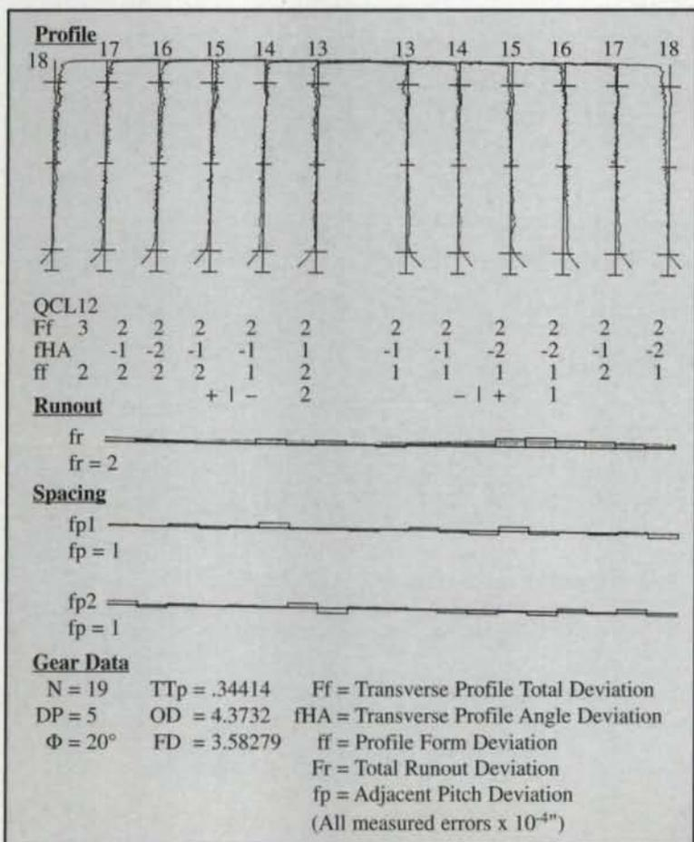
Fig. 11 — 5 DP wire EDM coarse-pitch gear data.
