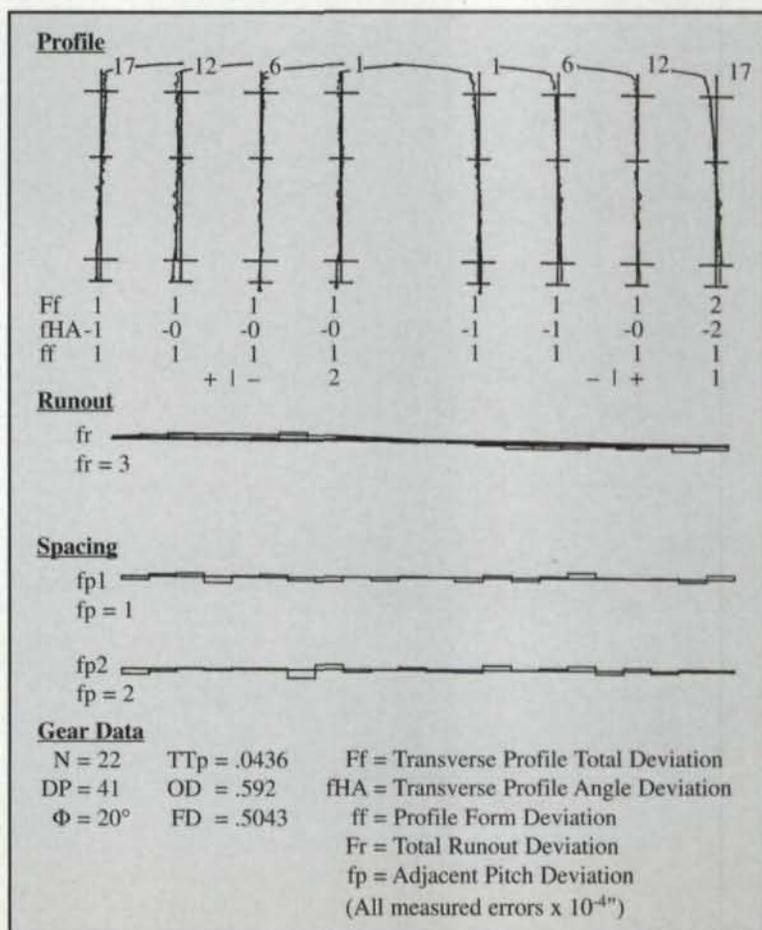
Fig. 9 — 41 DP wire EDM gear data.
