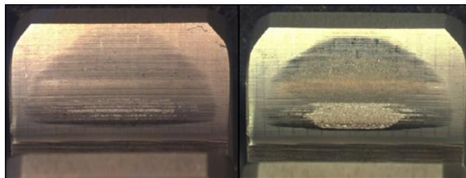
Figure 7—Tooth surfaces of a pinion operated at (left) SKS 9 after 40 hours and (right) SKS 9 after 160 hours. (Photos courtesy of Gearlab at The Ohio State University.)
