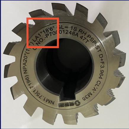
Figure 3—Hob marking for spur gear.
