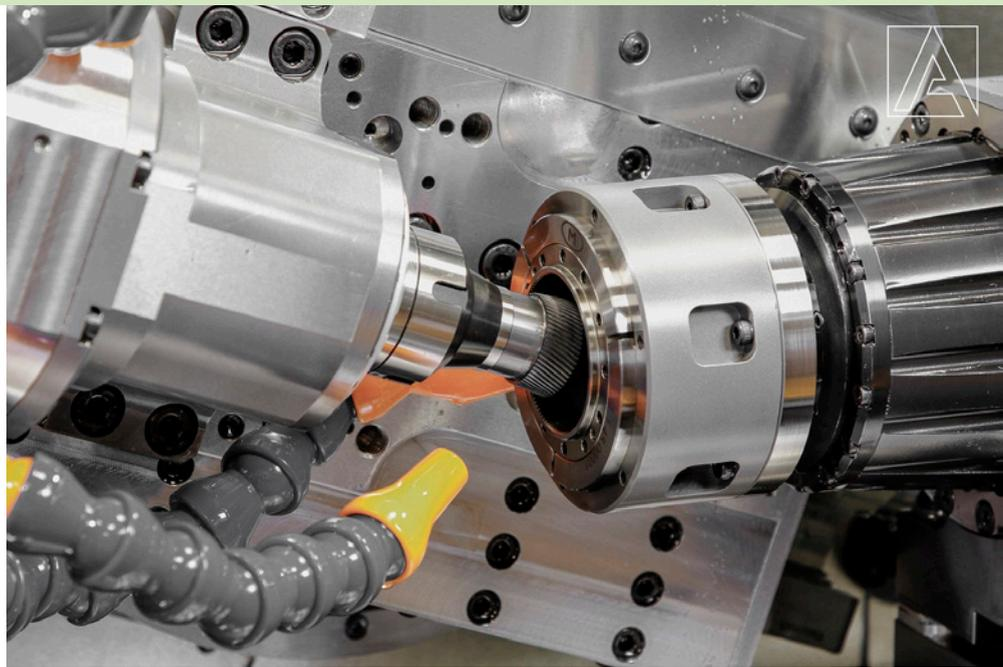
and the C prime axis is equipped with a driven spindle. Vincent Affolter: “This configuration is designed for the power skiving of internal gears. The production of face gears is possible, too.”
