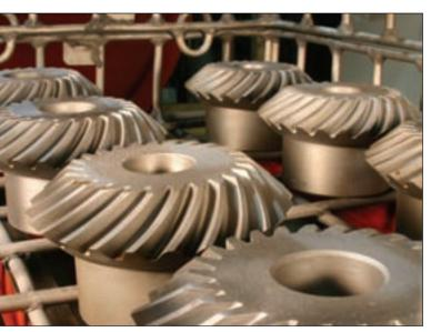
A tray of spiral bevel gears after vacuum carburization at Solar Atmospheres.
