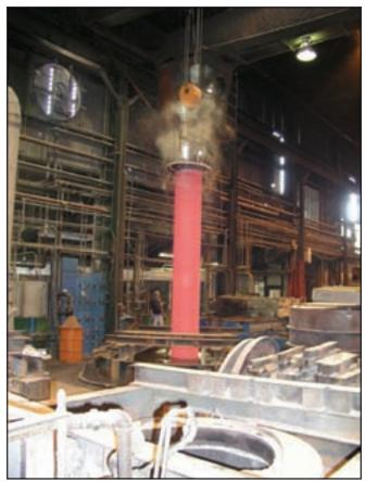
An in-process rope drum quenching at Xtek.
