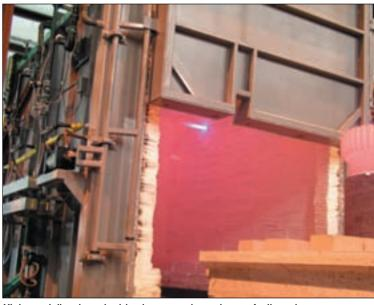
Xtek specializes in carburizing heavy equipment gears for its customers.
