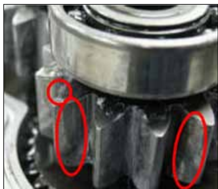
Figure 15—Damaged gear without crowning.
