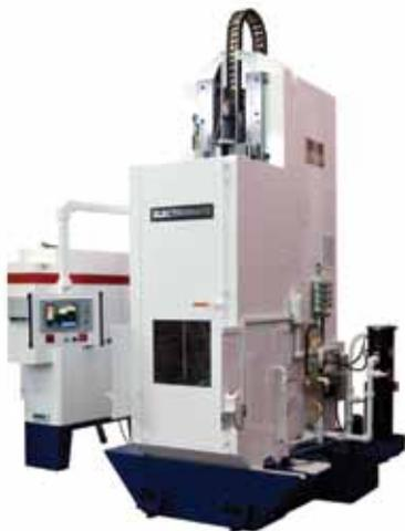
Modern broaching machines replace hydraulic systems with electromechanical systems, including servo drives and high precision ballscrews or planetary roller screws. Courtesy of Broaching Machine Specialties.
