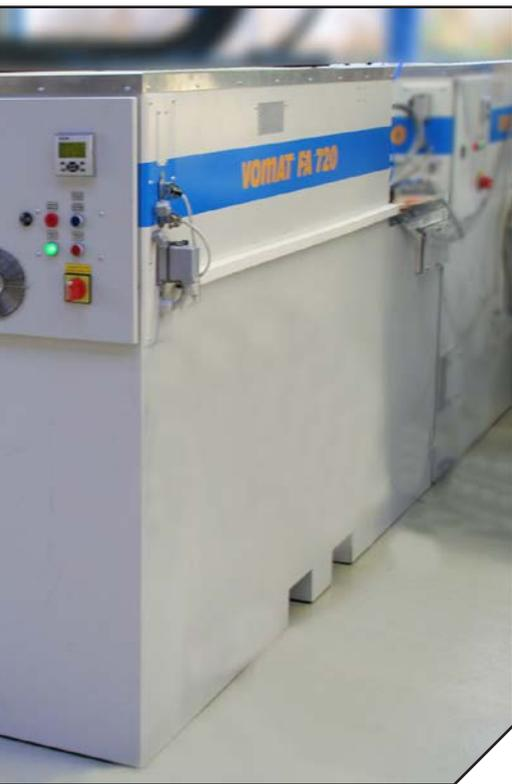
ing the backflush cycle the operator always has full oil flow. This allows for energy efficient, time optimized operation in sync with the customer's grinding machine. The Vomat FA 120 through 420 series machines with dimensions of 1 x 1 x 1.6 meters are also significantly smaller than comparable filtration systems on the market. This keeps transportation costs low, possibly reduces
