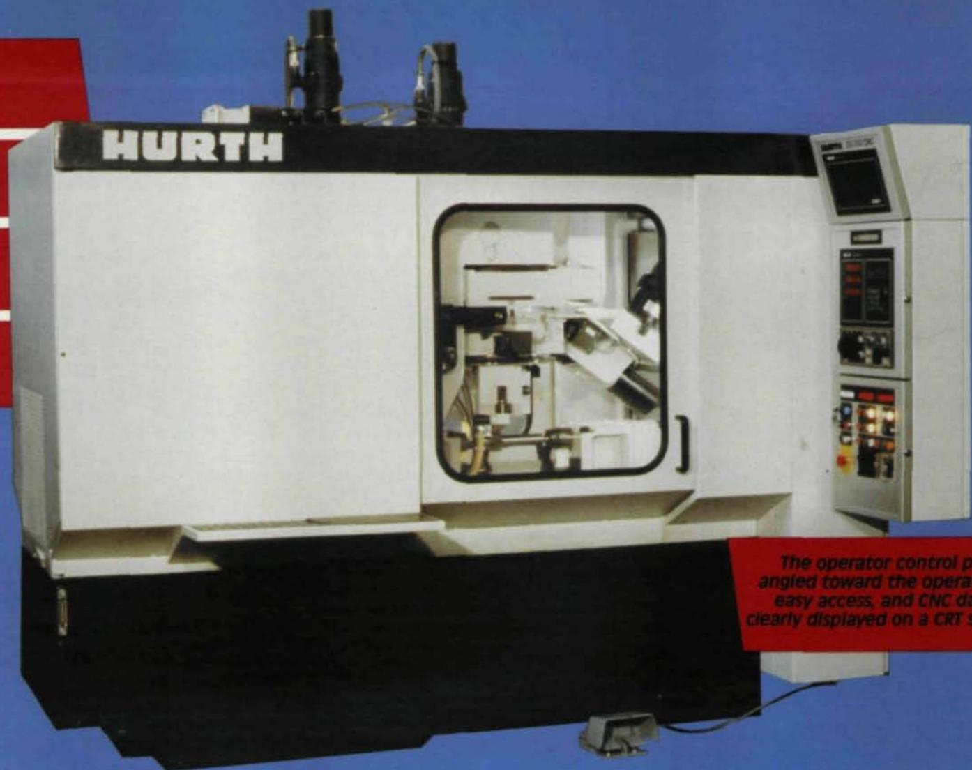
The operator control panel is angled toward the operator for easy access, and CNC data are clearly displayed on a CRT screen.
