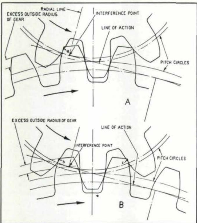
Fig. 12 — Diagram Illustrating Term Known as Involute Interference. Gear Tooth Contacts Non-Involute Portion of Pinion Tooth Outside the Zone of Contact.
