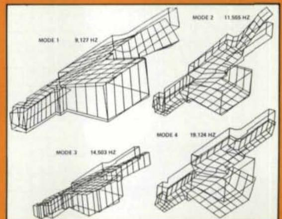
Fig. 13—(top right) Finite element model, mode shapes, and frequencies of modified ATS—Gear
