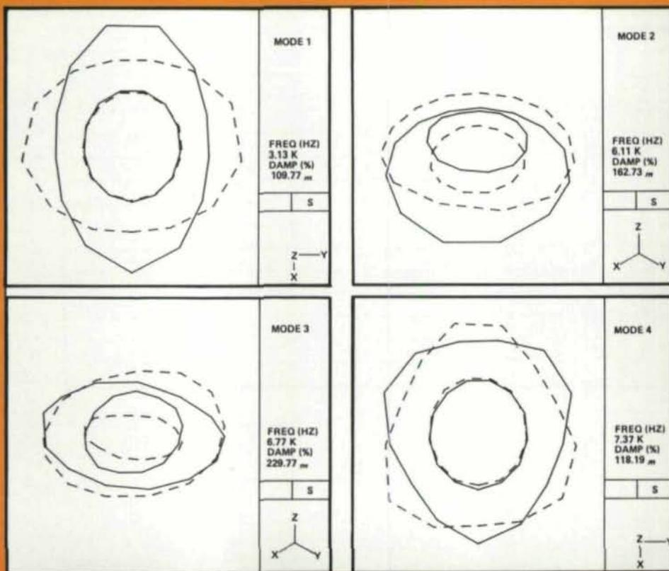
Fig. 11—(bottom right) Mode shapes and frequencies of baseline ATS—Gear
