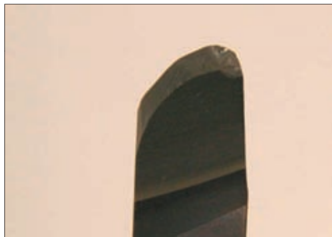
Figure 11—Large blade top chipping called “banana peel.”
