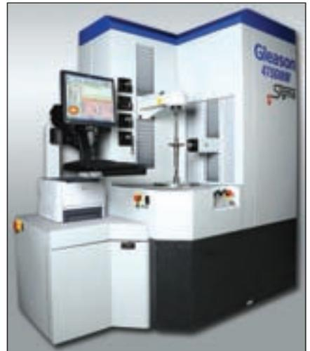
The Sigma 475 and 1500GMM Analytical Gear Testers provide complete bevel and cylindrical gear inspection featuring a three-dimensional scanning probe head. These testers are powered by new *GAMA* native software that covers a range of gear applications.
