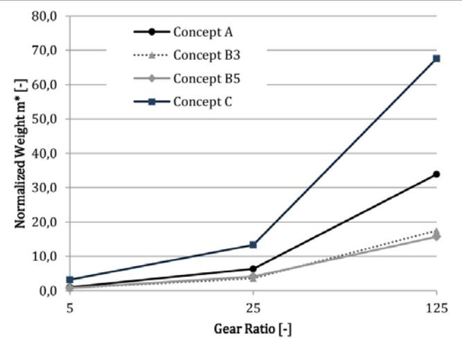
Figure 8 Weight of conventional and low-loss external gear.
