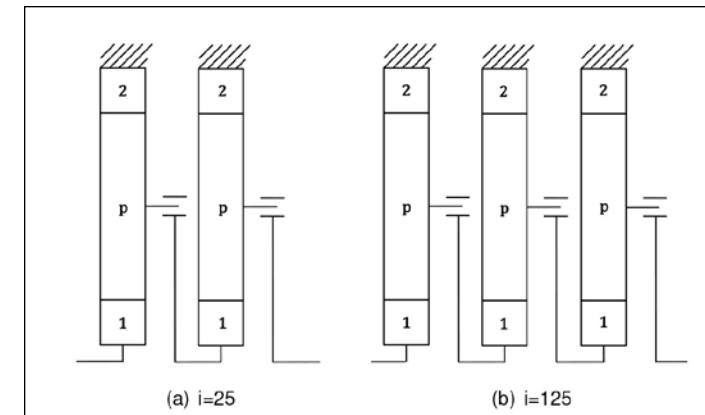
Figure 5 Concept A with gear ratio 25 and 125.
