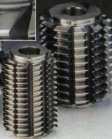
**P**recision hobs with a superb surface finish are the result of new production methods now in place at Star Cutter. Hardened hobs are finished by skiving or grinding, depending on hob geometry. The vast majority are skived, providing additional regrind life. The EDM process has been discontinued.
