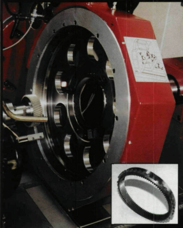
Honing of Automatic Transmission Ring Gear
