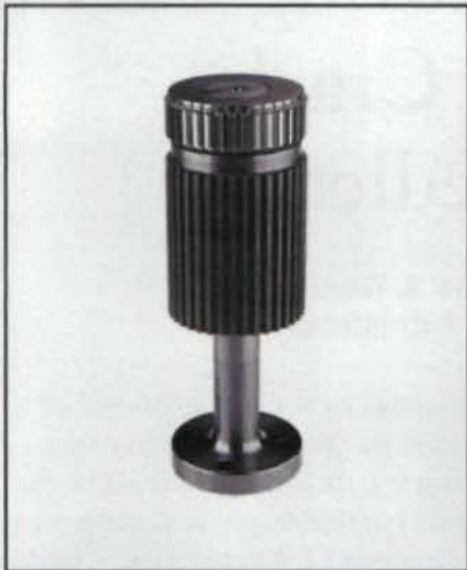
The short broach centers a gear with its upper set of teeth, then removes stock and flattens the gear's profile with the lower set of teeth.
