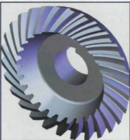
GearTrax 2003 has a new feature that can create 3-D models of spiral bevel gears for assembly drawings.
