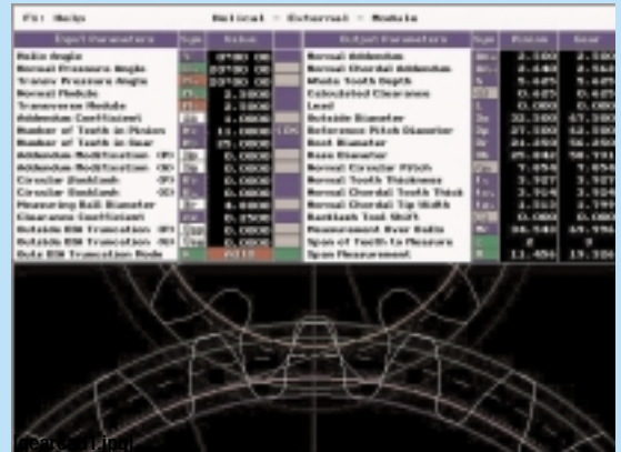
GearCAD is used for calculating internal and external spur, helical and planetary gears.
