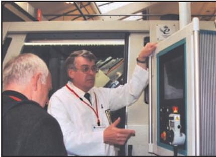
**Holroyd developed its own software and controls for the GTG2.**
