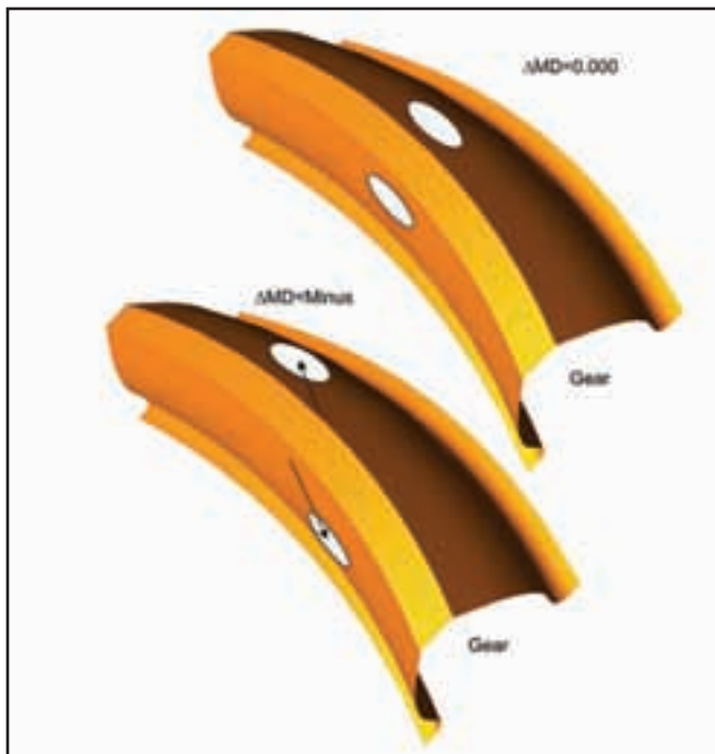
Figure 14—Changes in contact patterns with pinion assembled too close to ring gear.
