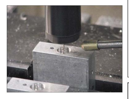
The Society of Manufacturing Engineers (SME) recently announced the release of Minimum Quantity Lubrication, an addition to the SME Manufacturing Insights Video Series. According to the organization's press release, the video surveys four different manufacturers that use MQL to apply only the minimum amount of lubricant needed for each job.
