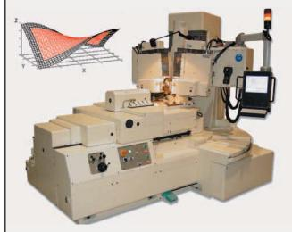
Advanced topological gear grinding, based on MAAG 0° grinding system.
