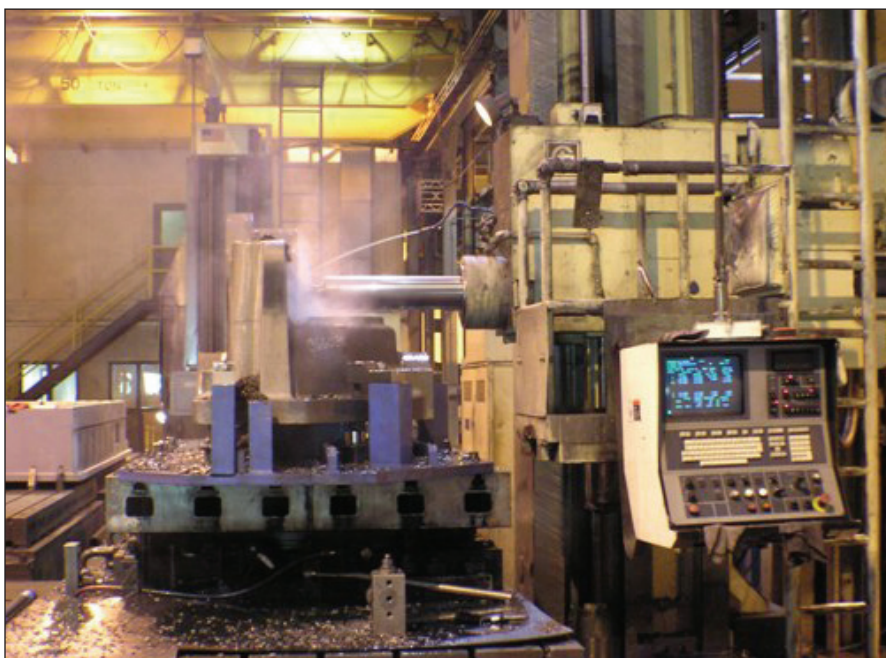
A look at an upper-gearcase component being premachined at Advance Mfg.
