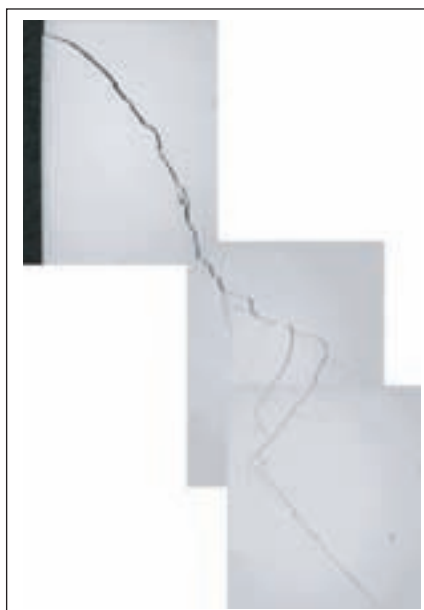
Figure 5—Photo montage of crack from tooth surface.
