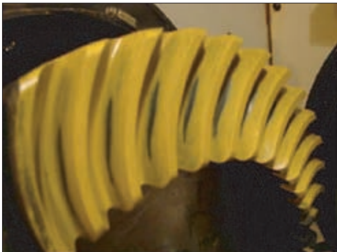
Figure 8—A typical contact pattern from field return.
