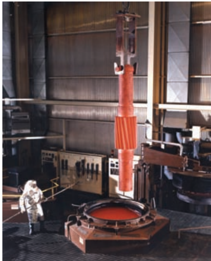
Heat treating is a crucial component in the manufacture of large gears and pinions. Photo/Rexnord.
