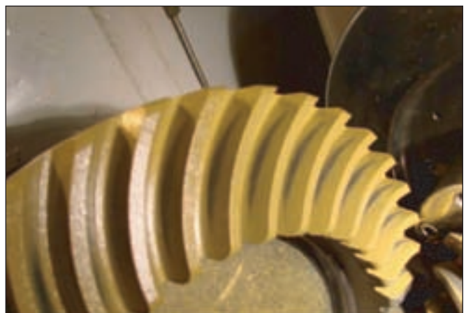
Figure 12—Post-test contact pattern between tested pinion and semi-master ring gear.
