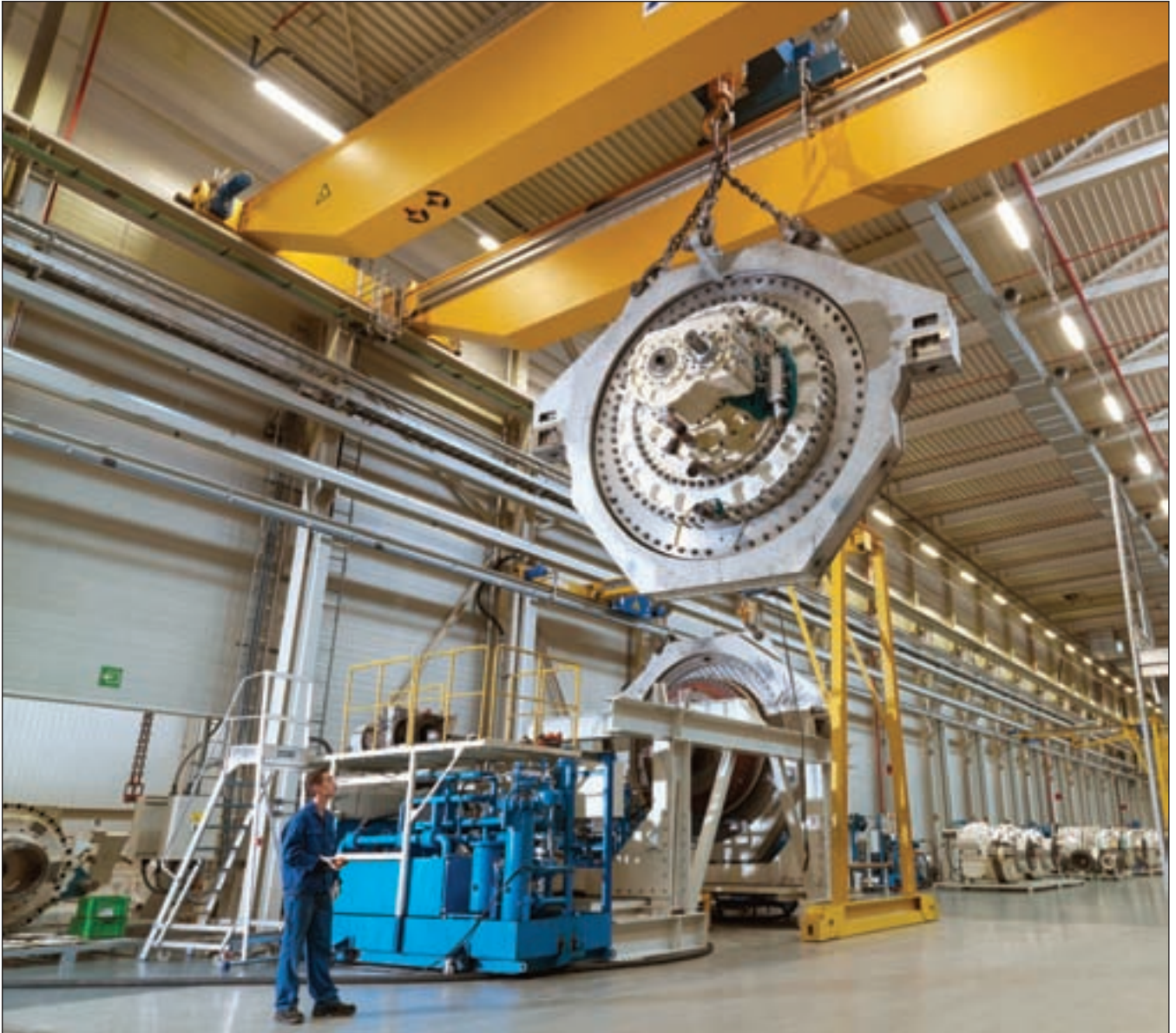
A wind turbine gearbox being moved at Hansen Transmission's Lommel, Belgium facility. Courtesy Hansen Transmissions.
