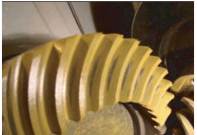
Figure 9—Post-test contact pattern from wear test sample.
