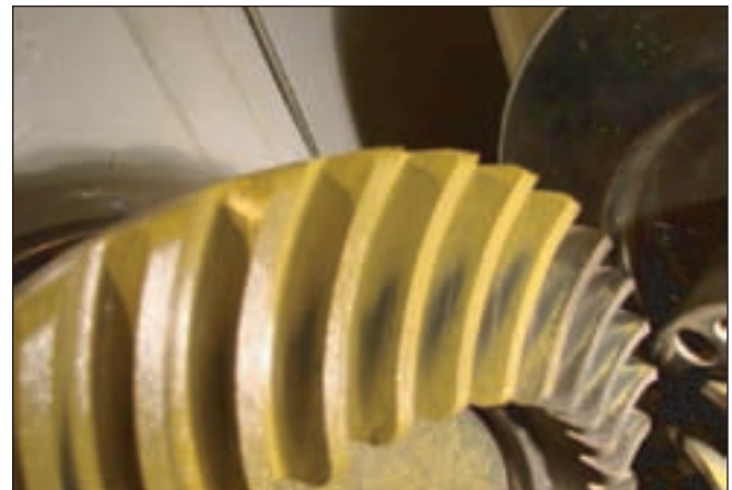
Figure 11—Post-test contact pattern between tested ring gear and semi-master pinion.
