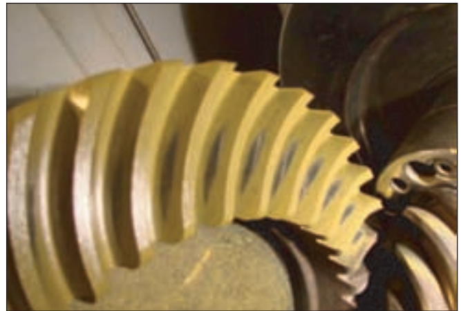
Figure 10—Post-test contact pattern from wear test sample with less severity.
