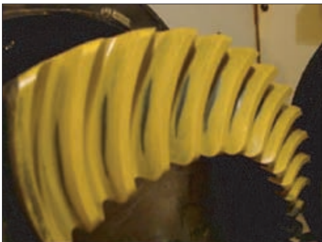
Figure 8—A typical contact pattern from field return.
