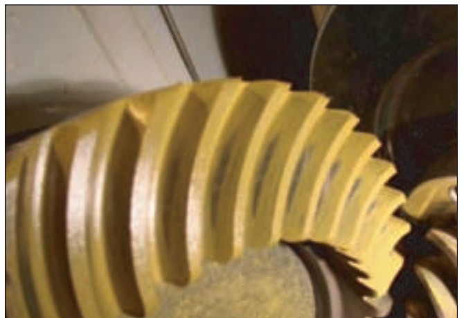
Figure 9—Post-test contact pattern from wear test sample.
