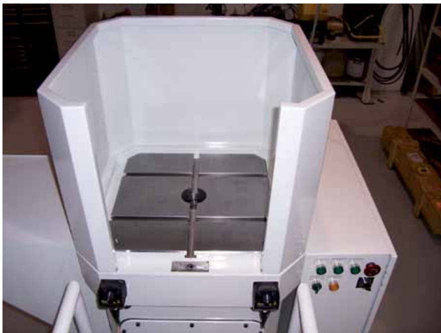
The table top design features crossing T-slots for faster and more accurate setups (courtesy of American Broach).
