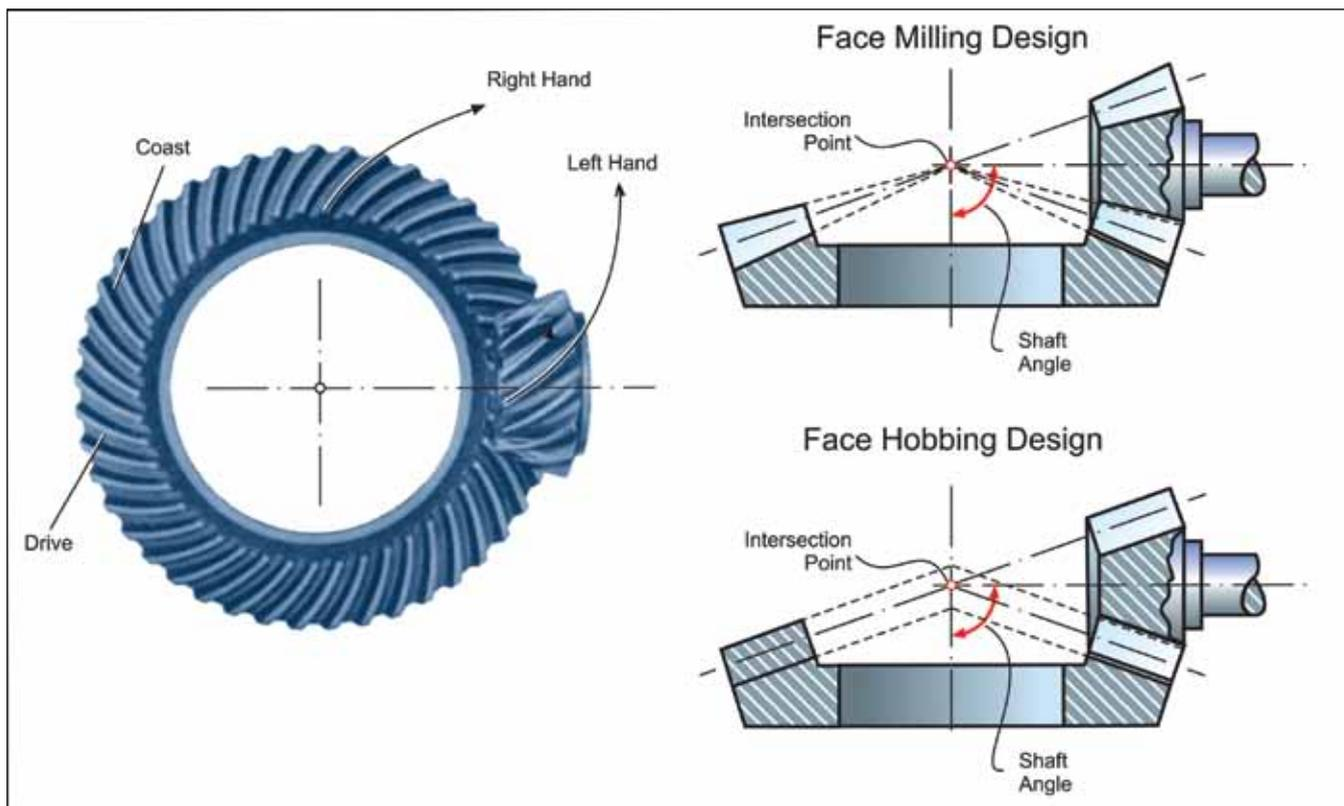
Figure 1—Spiral bevel gear geometry.
