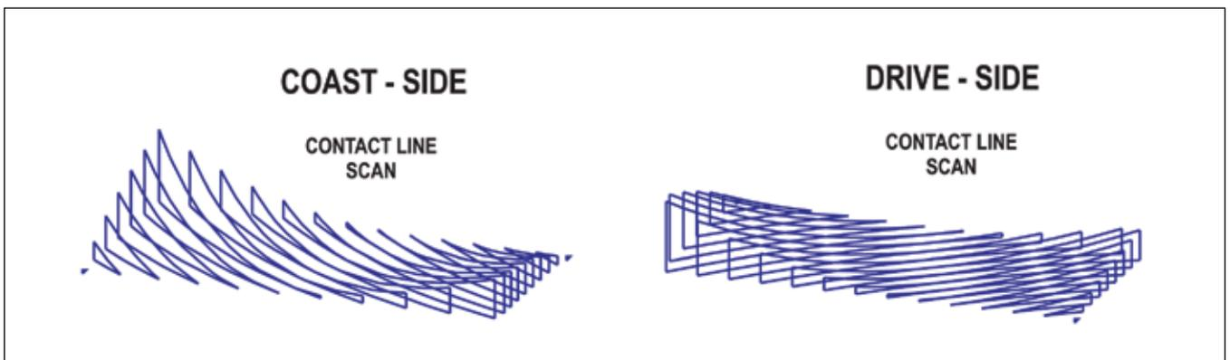
Figure 3—Contact-line scan of a spiral bevel gear set.
