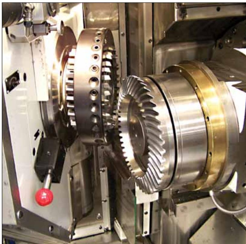
Figure 6—Spiral bevel gear cutting with face hobbing cutter (continuous process).
