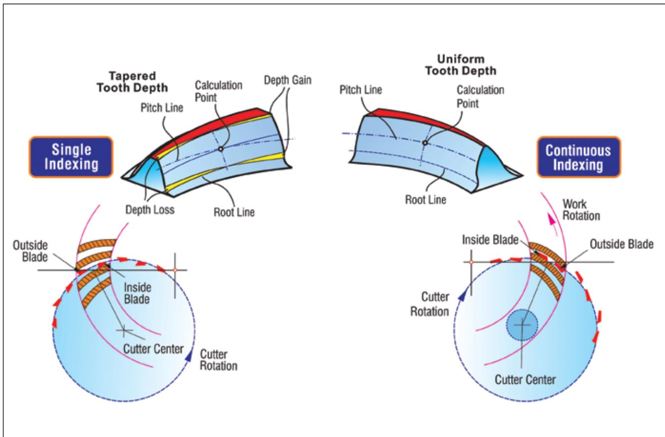
Figure 5—Left: face milling; Right: face hobbing.
