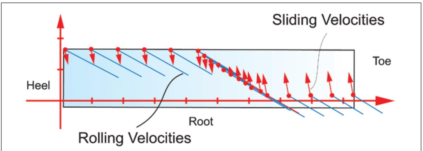
Figure 4—Rolling- and sliding-velocities of a spiral bevel gear set in path-of-contact points.
