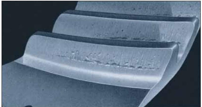
Figure 7—Pitch-line pitting on a spiral bevel gear surface.
