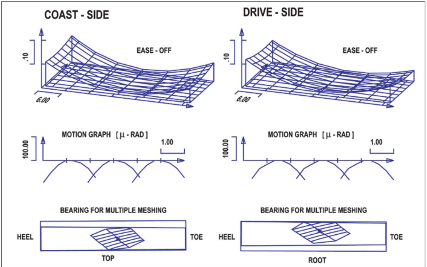
Figure 2—Tooth contact analysis of a spiral bevel gear set.
