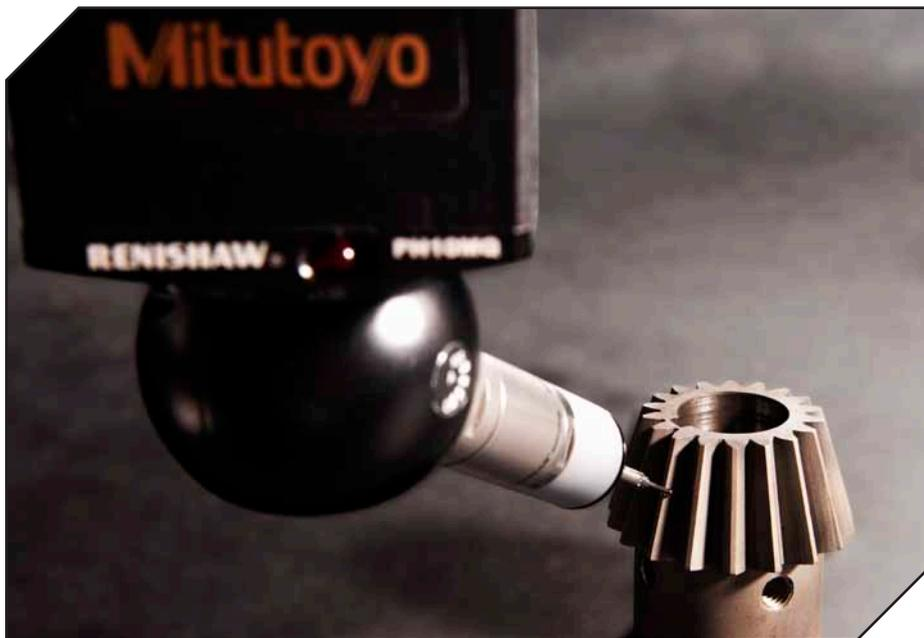
Fox says. By incorporating high-level software, CMMs can measure virtually any type of geometry. For example, airfoils, compressor scrolls or turbine blade geometry can be inspected with the appropriate software. In addition, “the ability to incorporate components such as vision probes using edge detection technology and laser line scanning probes have made CMMs much more flexible and powerful,” Fox says.
