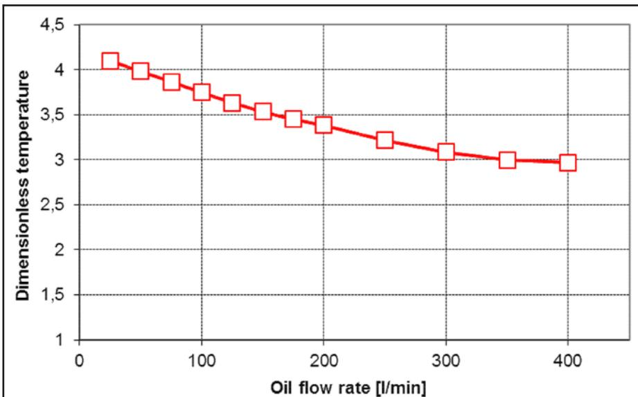
Figure 6 Evolution of gear wheel bulk temperature vs. oil flow rate.
