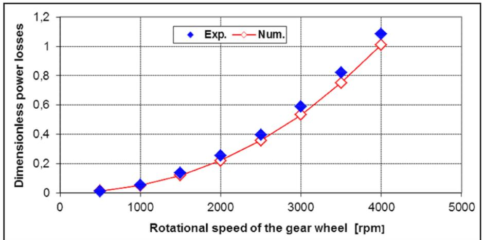
Figure 3 Dimensionless power losses vs. rotational speed.
