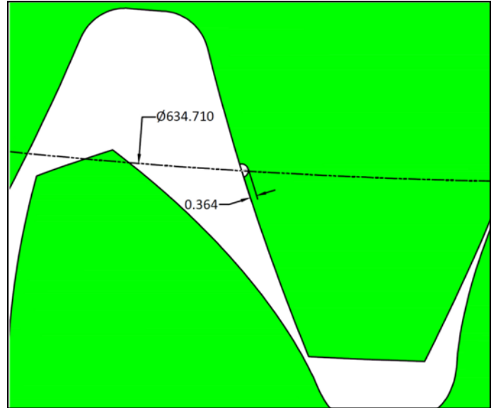
Figure 11 Detail of depth and position of pitting.
