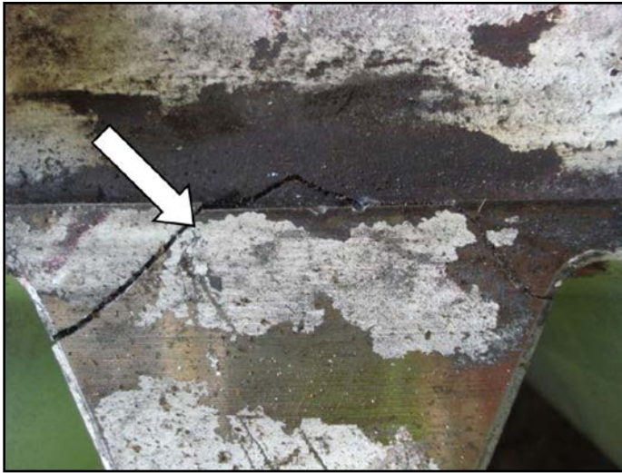
Figure 3 Tooth root crack due to misalignment.
