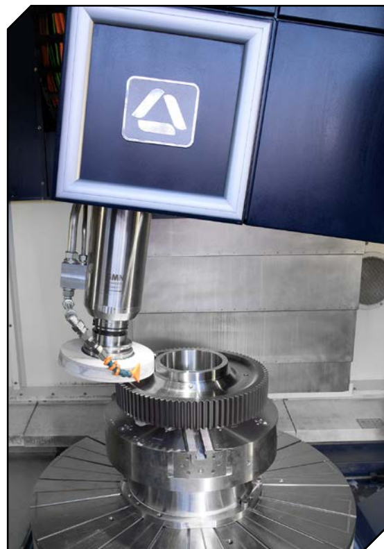
Danobat's customized gear grinding machines make it possible for Grupos Diferenciales to turn, grind and measure large parts.
