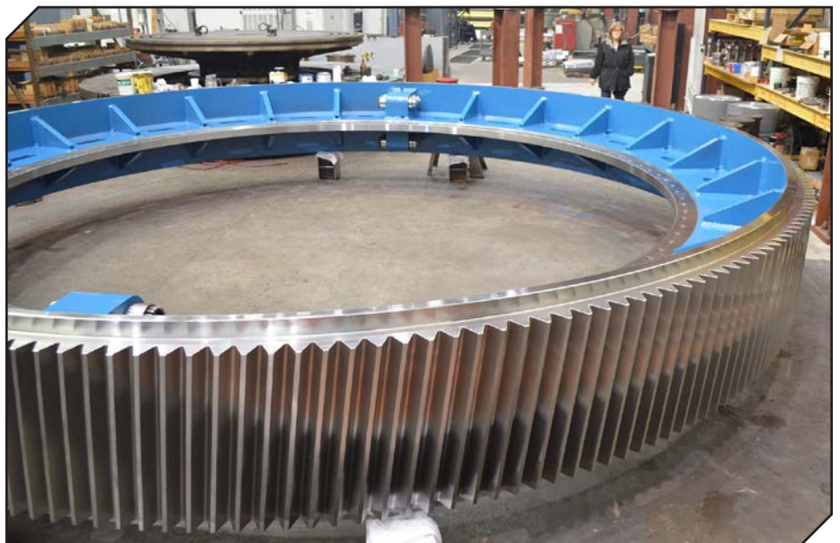
Recent upgrades in tooling and machine tool technology have made it easier to manufacture higher quality gears in 2019 (photo courtesy of HMC).
