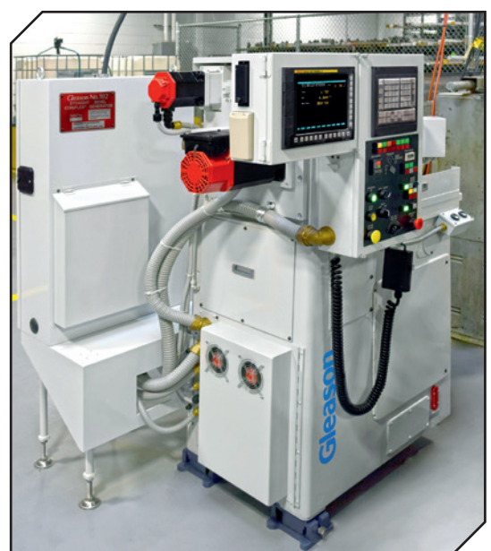
Figures 1, 2 (before and after) The Gleason Modernization Program is enabling SDP/SI to add Coniflex capacity by transforming its manual, 60s era 102 Generators into CNC machines that set up easier and run faster and more reliably.
