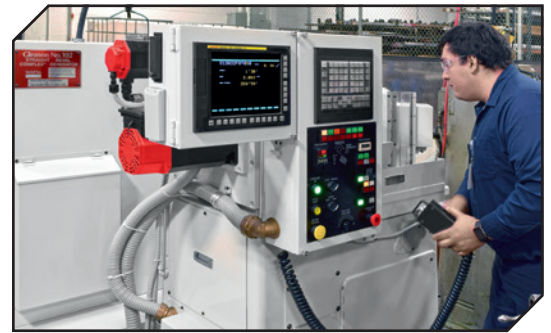
Figure 3 The 102 CNC Generator is far less dependent on an increasingly scarce pool of operator experience for setup and operation. The Fanuc CNC retrofit enables an operator with just a week or two of training to run the machine more productively and with far less time spent on setup.
