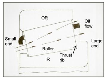
Figure 30-Lubricant flow in a TRB (Ref. 2).
