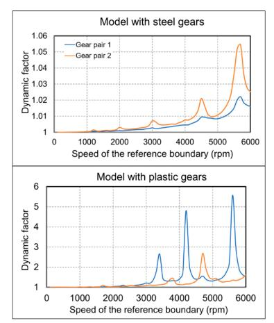
Figure 2-Dynamic factor without gear meshing damping, d=0 Ns/m.
