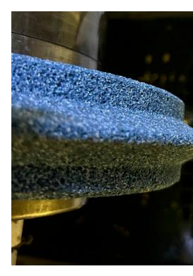
parameters in the profile grinding process can result in increased cycle time, poor gear quality, burning and increased scrap in gear production. Consulting with an application engineer, such as from an abrasives manufacturer like Weiler Abrasives, can improve results.
