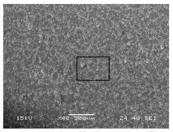
Figure 11-SEM image of the IR raceway at 40x magnification.
