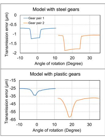
Figure 3-Transmission error of the gear pairs.
