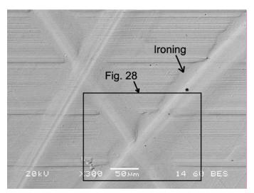
Figure 24-BSE image of the IR thrust rib at higher magnification.
