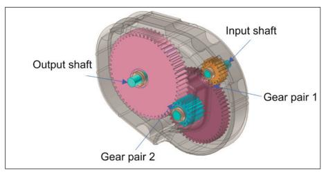
Figure 1-A two-stage gearbox model layout.
