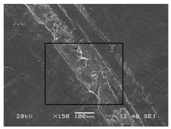
Figure 19-SEM image of roller end at higher magnification.
