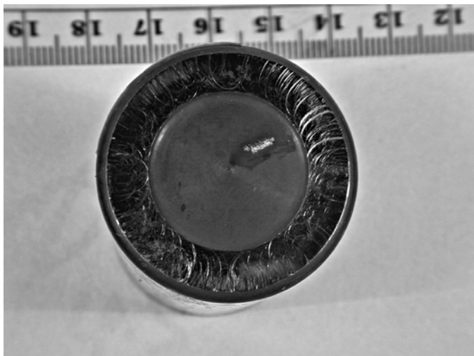
Figure 6—LOM image of the roller large end with a multitude of scratches.
