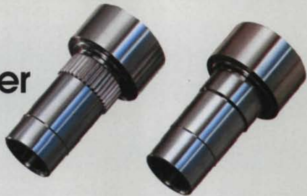
External blind splines are broached to within 0.0005-in. concentricity to internal bore.
