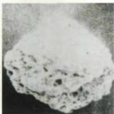
ALUMINUM OXIDE GRAIN
