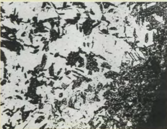
Fig. 2—Microstructure of a 2 DP final drive pinion which failed after 900 hours because of pitting.
