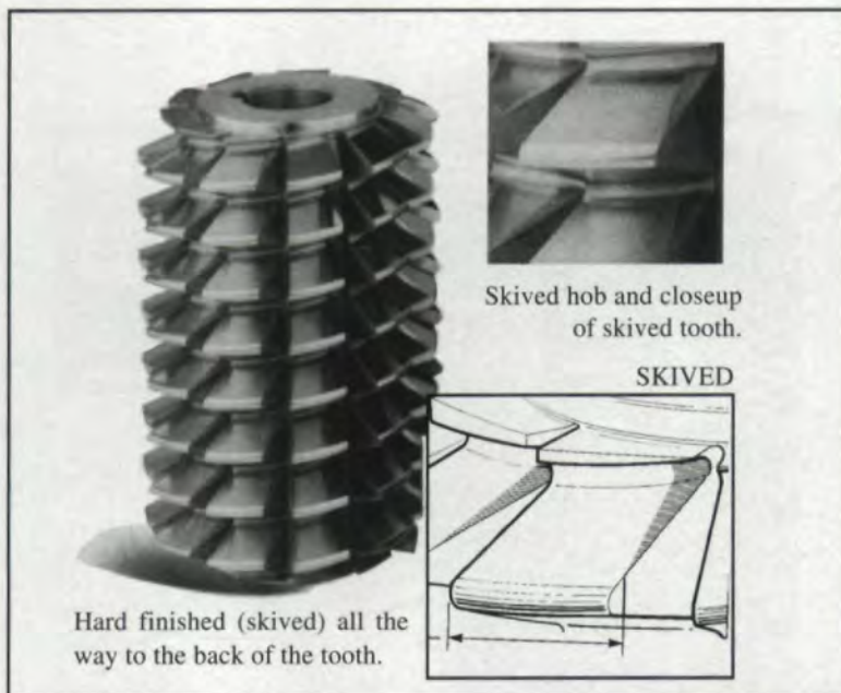
Fig. 3 - Skived finish hob made by Star Cutter. (Courtesy Star Cutter Company.)
