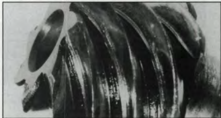
Fig. 14 - Excessive wear of a spiral pinion. We note the presence of steps in the profile root and pointed tooth tips. This pinion is near the end of its life.
