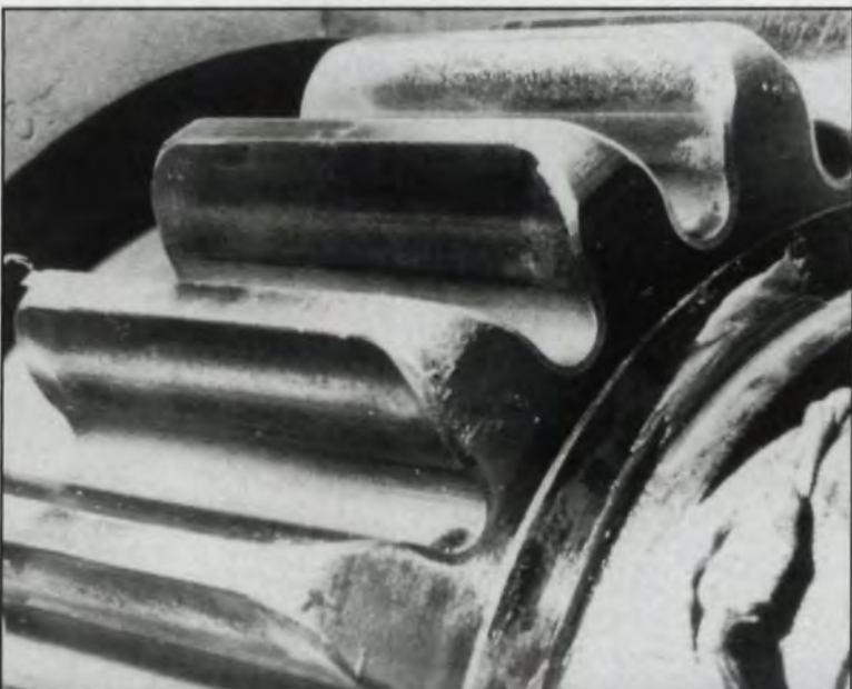
Fig. 11 - Moderate wear. We will note the trace of the operating pitch line on the teeth flanks and the presence of fine streaks indicating that the teeth operate near the limit rate of lubrication.
