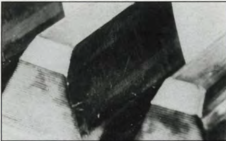
Fig. 9 - Normal wear. Aspect of a large gear wheel flank lubricated with grease.
