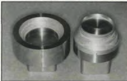
Fig. 8 — Fracture surfaces of 30° interlayer torsion specimen after testing.
