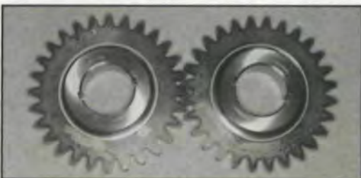
Fig. 10 — Pair of multi-metal fatigue test gears.
