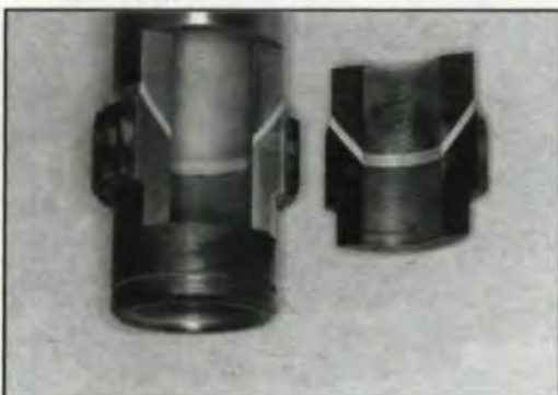
Fig. 17 — Segment removed from spline end of D6ac multi-metal sun gear for metallurgical evaluation.
