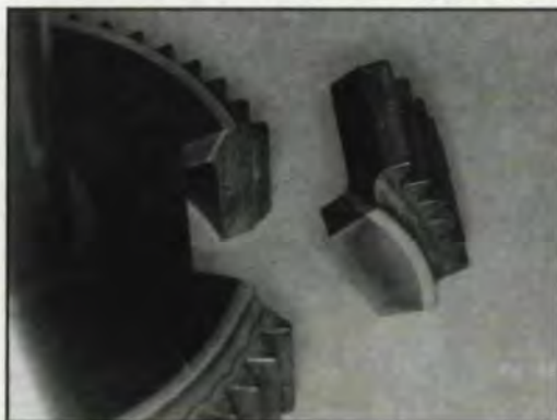
Fig. 16 — Segment removed from spur gear end of D6ac multi-metal sun gear for metallographic evaluation.
