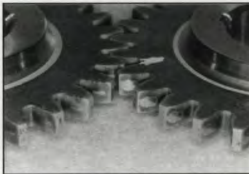
Fig. 11 — Contact surfaces of multi-metal fatigue test gears after testing.
