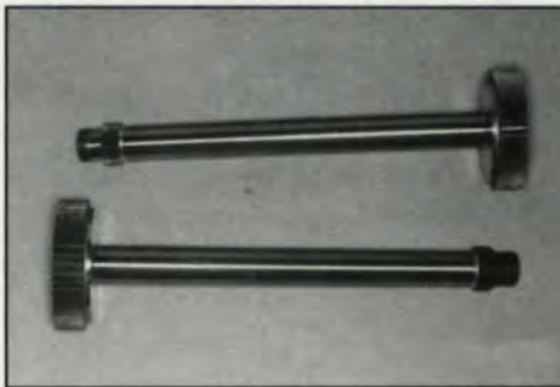
Fig. 13 — Multi-metal demonstration sun gears with gear and spline portions composed of 9310, top, and D6ac, bottom.
