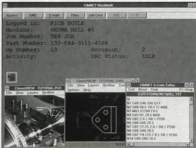
Graphic viewers provide MICS users with documents, drawings and digital photos at their workstations. Electronic folders may access any pertinent information on the network.
