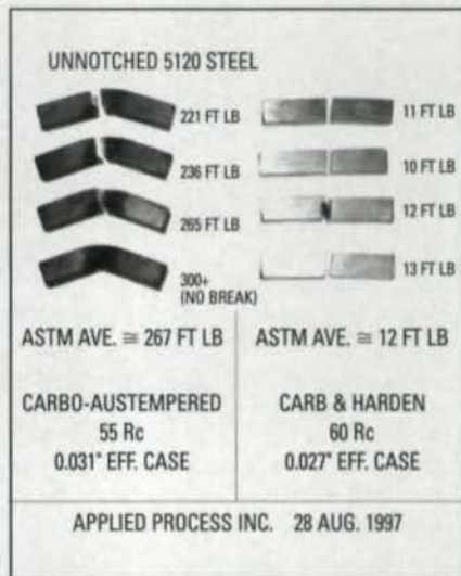
Fig. 30—A comparison of fatigue strength of unnotched Carbo-Austempered™ and carburized and hardened steel of similar hardness.
