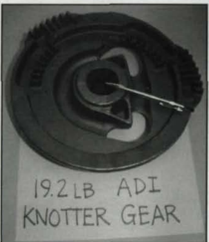
Fig. 21—ADI hay baler knotter gear.
