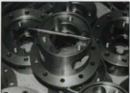
Fig. 20—ADI limited slip differential gear housing.
