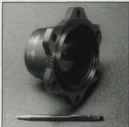
Fig. 18—ADI inboard constant velocity joint for light vehicles (Courtesy of Delphi).
