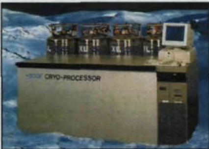
This machine lowers a gear's temperature by less than 1° per minute.
