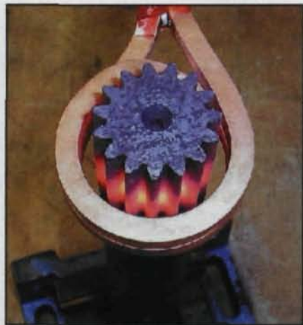
On a shaft, a spur gear pattern is induction hardened by a medium frequency and a high frequency transmitted at the same time via an induction hardening system from Electroheat Technologies L.L.C.
