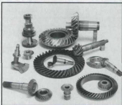
Spiral & Straight Bevel Gear Manufacturing.
