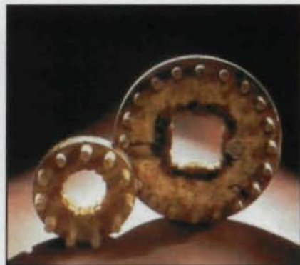
These antique gears at The Smithsonian Institution’s “Engines of Change” exhibit are constructed with five species of wood.
