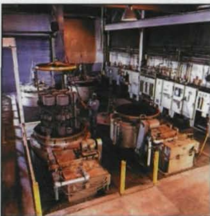
Figure 7—A load of diesel engine gears is removed from the furnace after nitriding.
