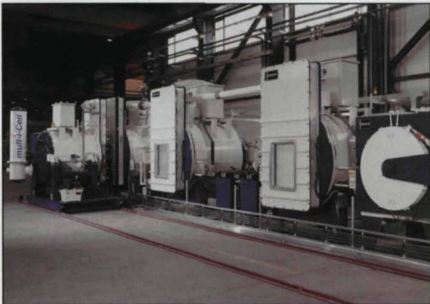
New from Ipsen International Inc., multi-i-cell includes a mobile vacuum loader (far left) that moves on rails in front of process and quench chambers.
