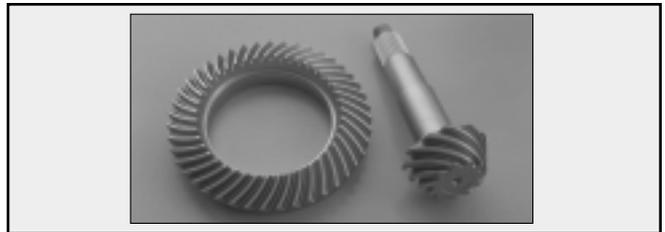
Figure 11—Ring gear and drive pinion.
