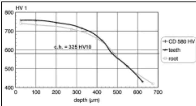
Figure 14—Hardness profile of 16MnCr5 gear wheel.
