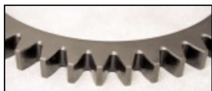
Figure 4—View of gear teeth with uniform chamfer as produced by chamfer hob.
