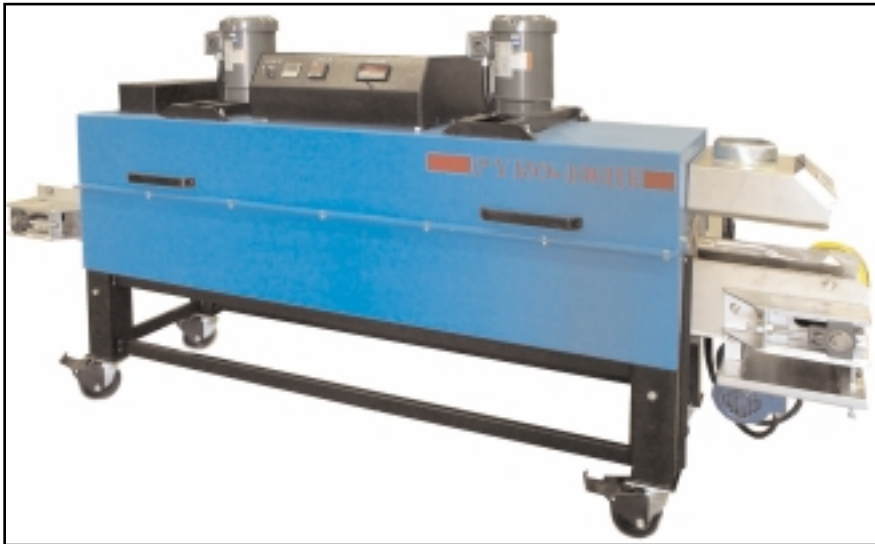
The Pyro Try Out oven from Pyromaitre is used for stress relieving spiral bevel ring gears.
