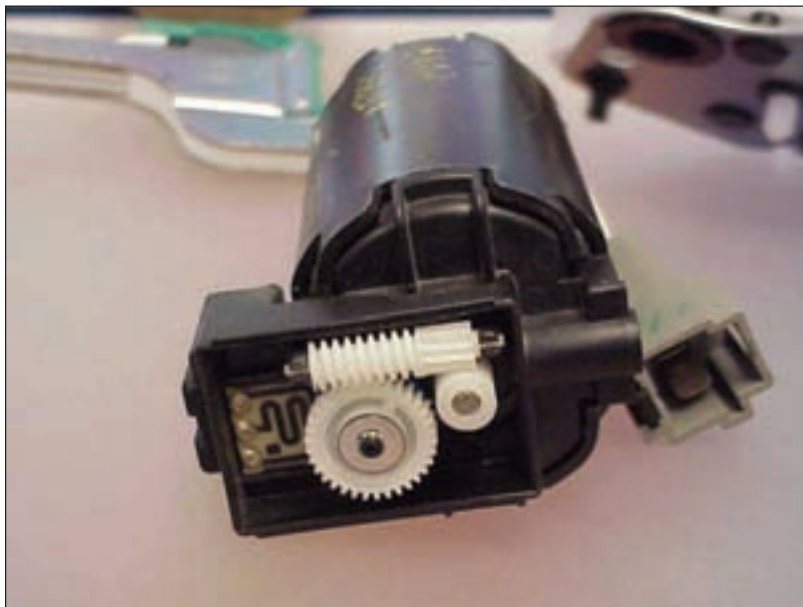
Plastic gears are now common in automotive applications such as this seat position sensor from ABA-PGT.
