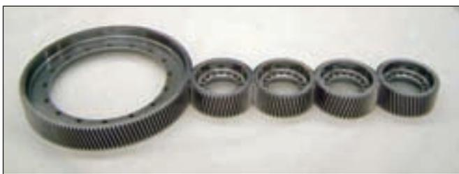
Figure 8—Entire gear train after superfinishing.
