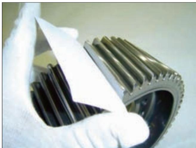
Figure 9—Close-up of a superfinished gear.
