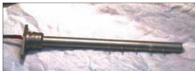
Figure 4—Photograph of thermocouple rake used in these tests.
