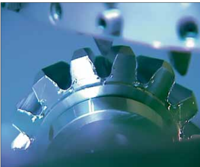
Figure 5—Bevel gear cut in the Hypoflex process.
