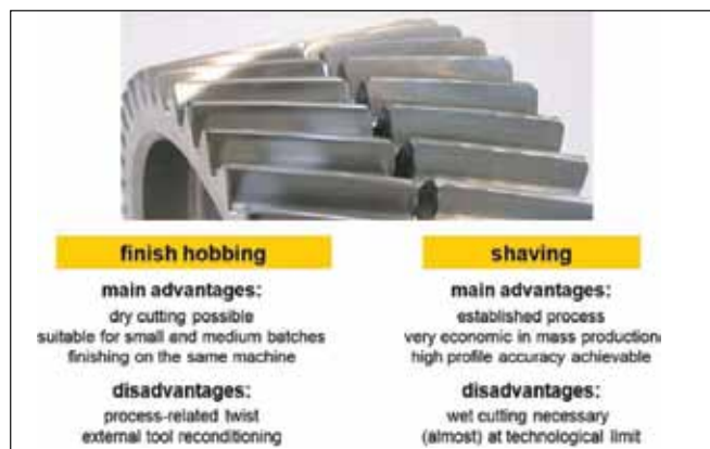
Figure 16—Finish hobbing versus shaving.
