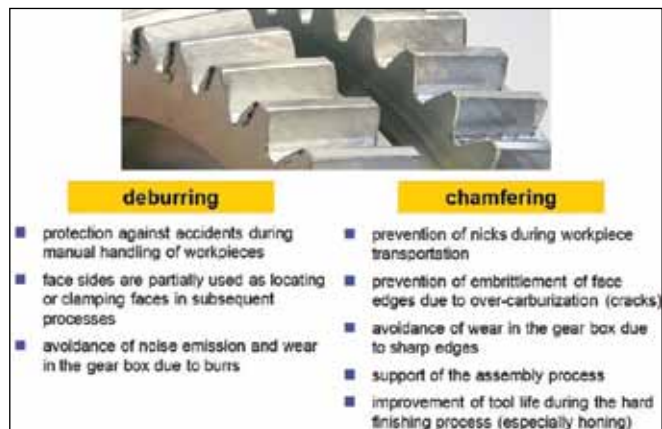
Figure 7—Why chamfering and deburring.
