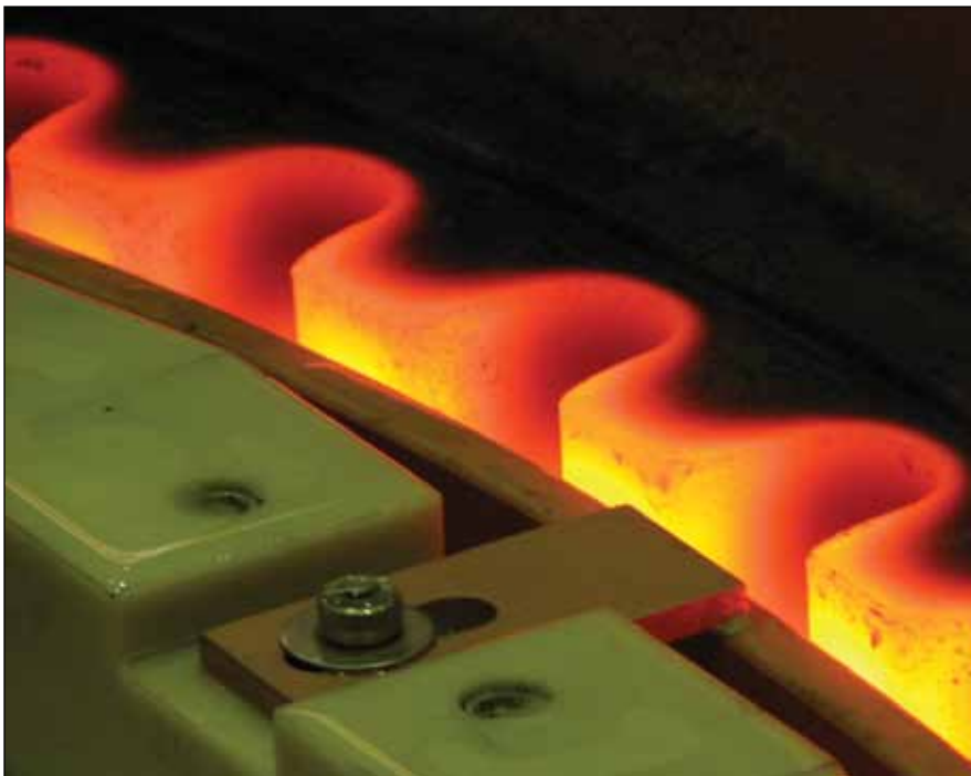
Induction Heating a large Caterpillar gear for hardening (courtesy of Caterpillar, Inc. and Ajax Tocco Magnethermic Corp).
