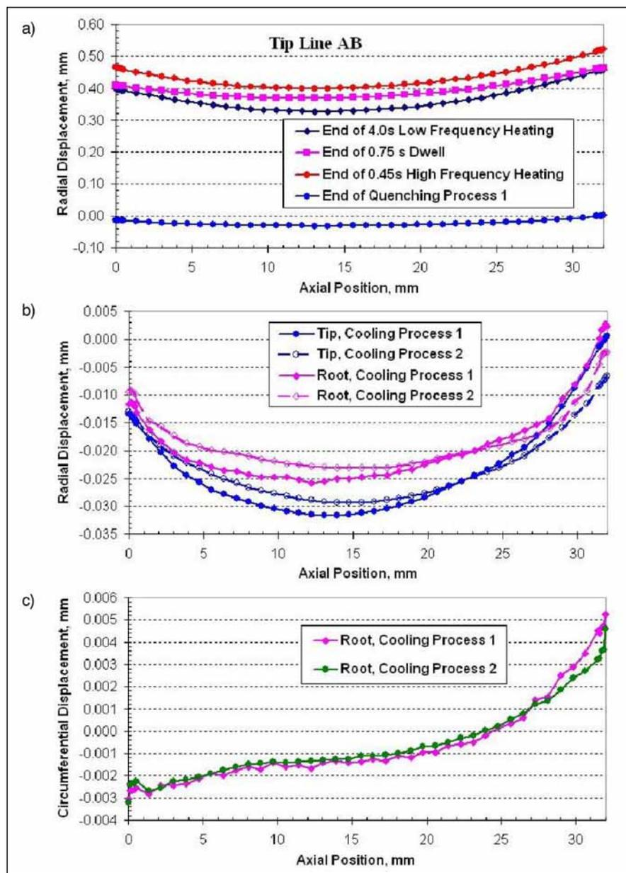
Figure 10—(a) Radial displacement of the gear tip line AB at different stages of heat treating processes; (b) radial distortion at the end of quench; (c) gear tooth unwinding distortion.
